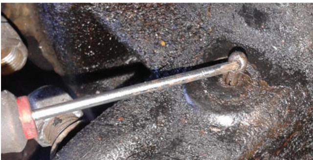
Picture 2: Relief valve split pin pulled free to move
